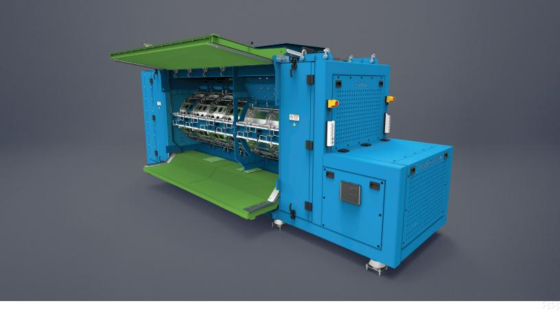
With the push of a button, the CleanREX opens for easy cleaning and faster service.
